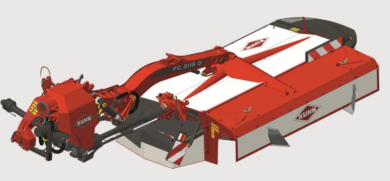
The FC 3115 D mounted mower conditioner complements KUHN's mower conditioner range with a working width of 3.10m and vertical folding system. Designed for forage farms and contractors, it can be used in combination with a front-mounted mower for higher work output. .
